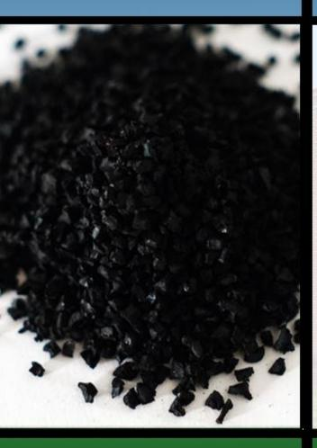
•grinding tyres in ambient temperature – tyre chips are size reduced with the use of mills, granulators and presses.
